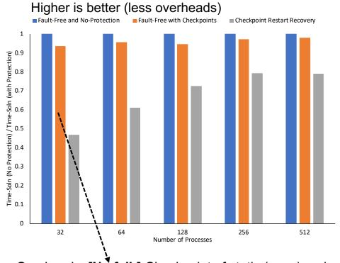
Overheads: [No fail:] Checkpoint of static (once) and dynamic states; [Failures:] No fail + state recovery, recompute, checkpoint (static, dynamic) state spares.
