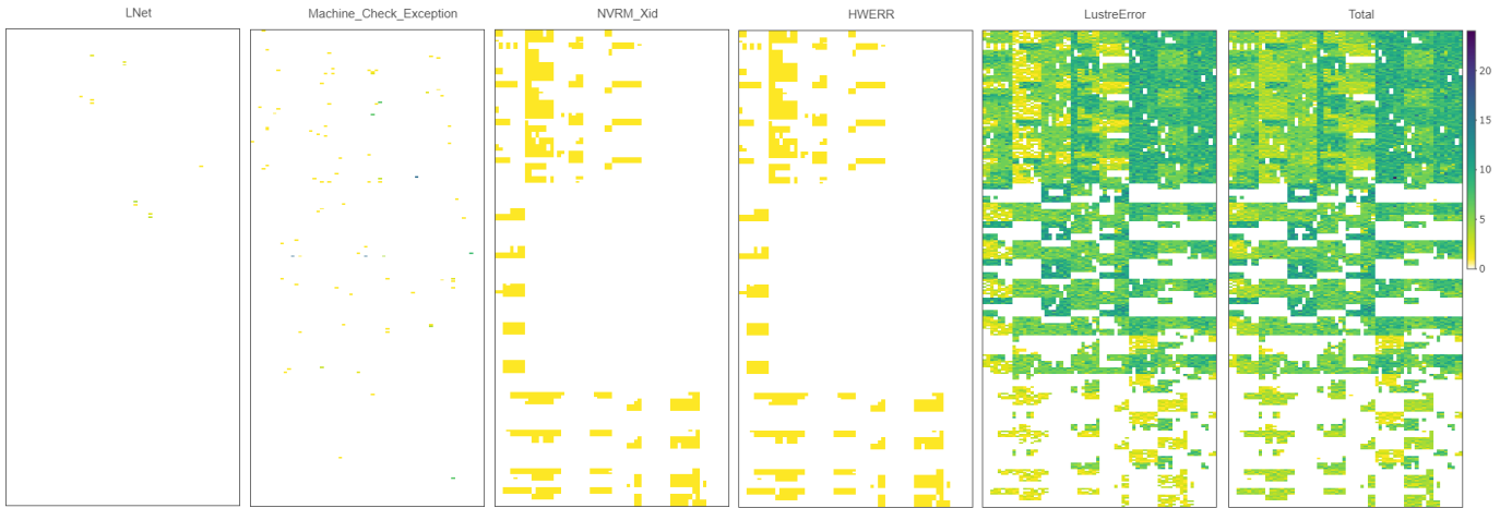
Fig. 2: The nodal layouts for every event type and the combined total for the past hour prior to “2015-02-09 01:49:54”. Each layout has dimensions of [300, 64] in pixel and each pixel represents a unique Titan node with its coordinates [X, Y] translated from its source name via Equation 1. The count numbers are plotted with common color bar with a top taken from the maximum total counts among all nodes.
