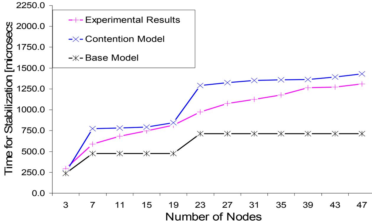
1. The model approximates the observed performance for a fully formed tree
