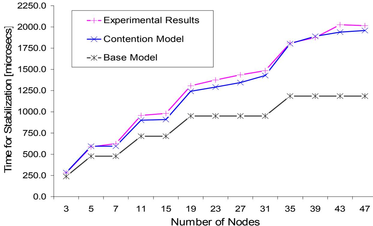
1. Base model shows step curve with increase in stabilization time
