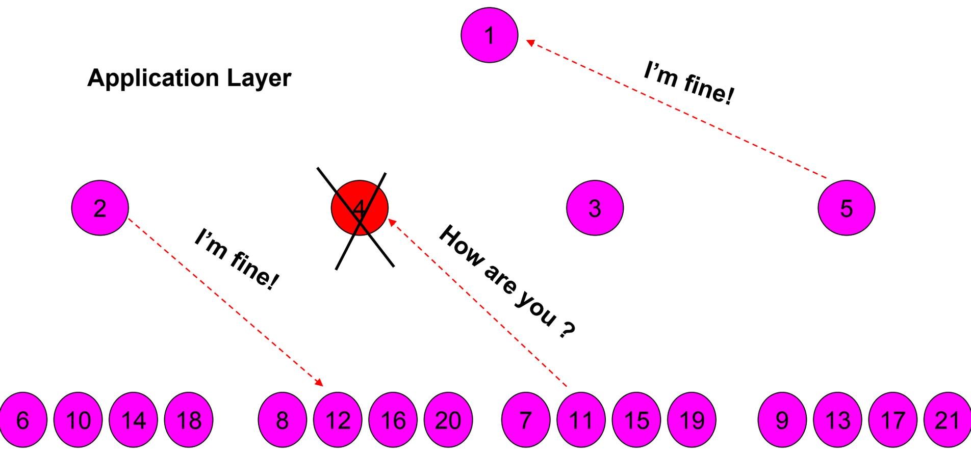
**Node 11 detects failure**
